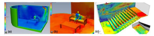
Figure 5: Example of PMV value and velocity slice place (a) and PPD result (b) of thermal comfort simulation result: (Autodesk Simulation CFD 2013) and Example of surface irradiation (c) of main lecture room: (STAR-CCM+ Building services 2013)
