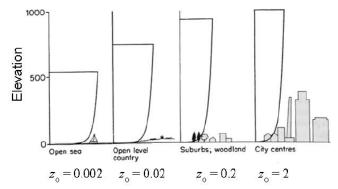
Figure 1: Mean wind profiles for different terrains: (P. Mendis 2007)
