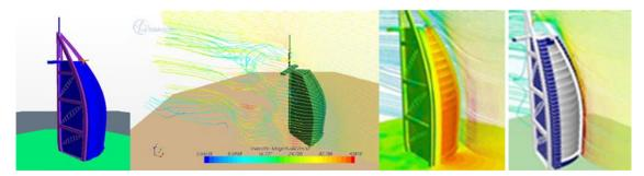
**Figure 2**: Velocity and pressure distribution create wind loading on building structure: (STAR-CCM+ for Building Services Analysis 2011)
